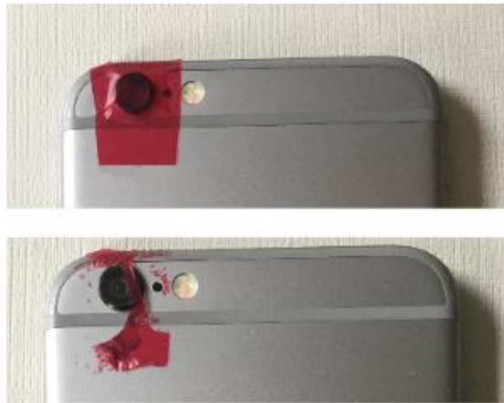
Figure A2: Sealed smartphone camera (intact and broken)
