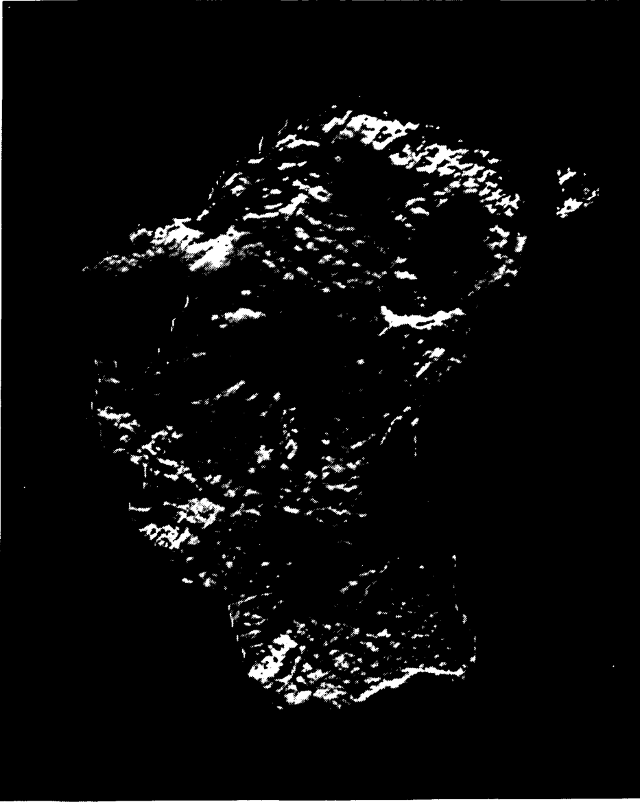
Topographic elevation data of Australia on a 6 minute (11 km approximate) grid displayed as an image and processed to give the impression of being illuminated from the west (digital east-west difference image). Such an image gives a good representation of the topography of Australia.
