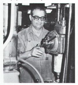
Drilling a sub-assembly for bit brace manufacture
