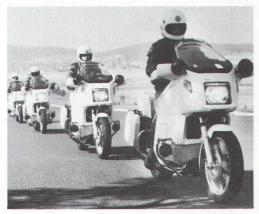
The BMW K100s used by the Force are specially modified for police work. They have a top speed of 215 kmph and their low mass and centre of gravity give them safe handling, even at these high speeds.
